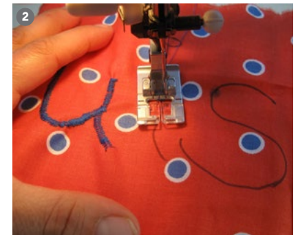
Stitch along the marked lines with wide, closely spaced zigzag stitching. Press stitching flat.
